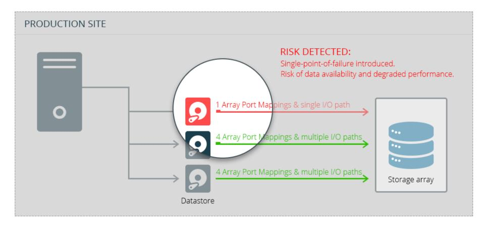
A datastore managed by a VMware ESX host is connected to SAN volumes with 4 I/O paths on different Host HBAs and ports, SAN fabric switches, and storage array ports to provide full redundancy and high performance.
