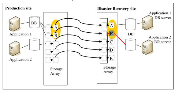
In this simplified configuration, application server 1 is running a database stored on 2 SAN volumes - A and B. RecoverGuard identifies these 2 volumes as constituting a data set used by Application 1. It then follows the replication path to determine that volumes A' and B' match the replica set. As seen above, it is evident that volume B' is incorrectly mapped to the wrong server, in this case, Application 2 DR server.
